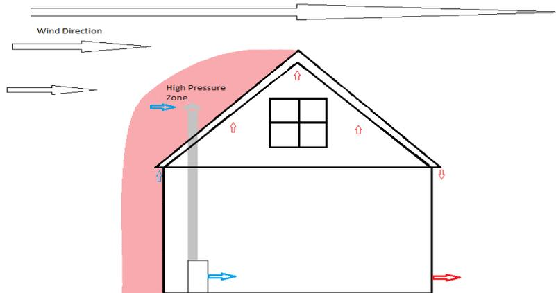
Firstly, all modern roof spaces have to be provided with roof ventilation and this often done by holes or grilles in the soffit boards. In strong wind conditions this can feel like a gale blowing across your loft. This can extract air from the building via light fittings and loft hatches. This effect can be mitigated by reducing the number of openings on the leeward side of the building, or again by balancing the upstairs pressures in the building independently from the ground floor.
